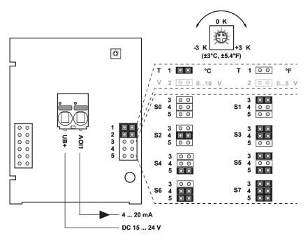
The adjustment of the measuring ranges is made by changing the bonding jumpers. The output value in the new measuring range is available after 2 seconds.
